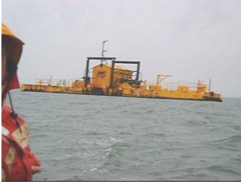
Fig. 2 Hydam – McCabe Wave Pump (SEI site visit to Carrigaholt Bay, Co. Clare, January 2004)
