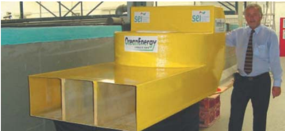
Fig. 1 Ocean Energy - Backward Bent Duct (scale model before delivery and testing in France (2004))
